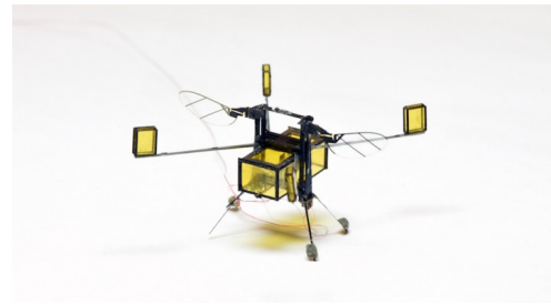
Figure 3 (a) Imperial College London's SailMAV with wings upturned to act as sails [5]. (b) Harvard University's microbot, with electrolysis chamber in yellow [6].
