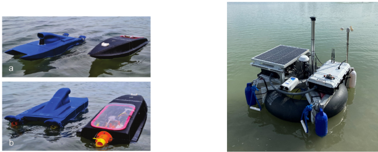
Figure 1 (a), (b) Front and rear view of New Dexterity's speedboat prototypes, showcasing 3D printed waterjet nozzle [1]. (c) University of Texas' USV with solar panel and bathymetric sensors [2].
