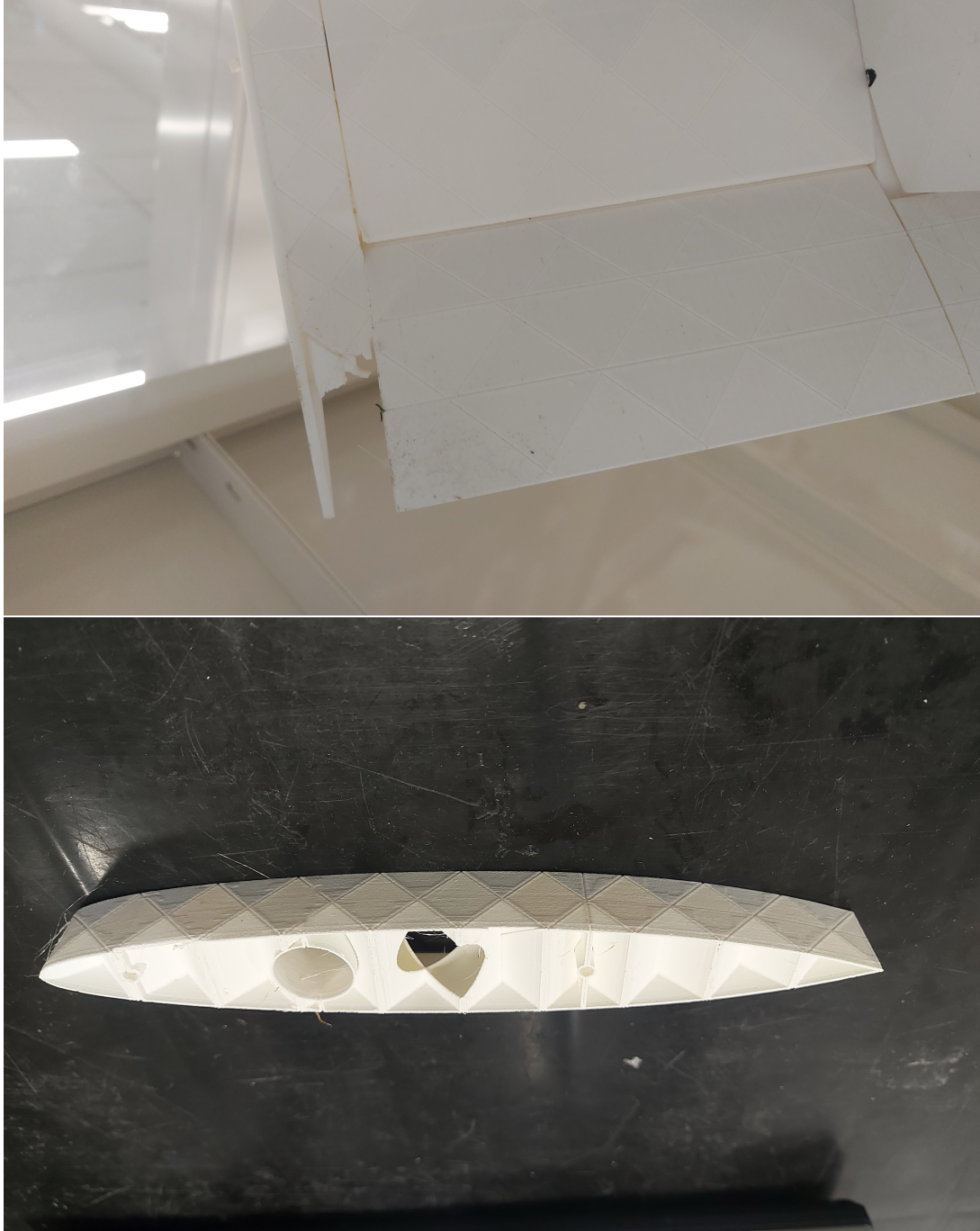
Figure 8 (a) Damage to the tail after a crash landing. (b) Replacement tail part, printed on a Prusa Mini using LW PLA.
