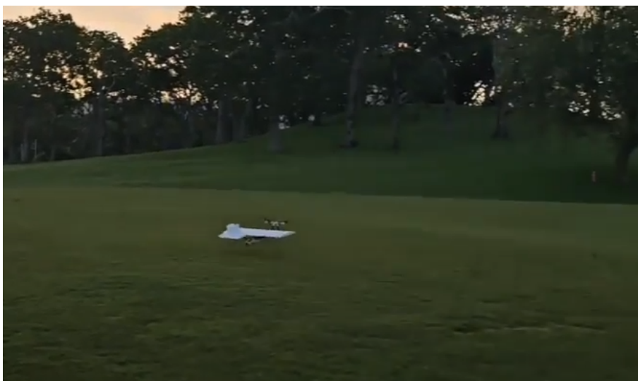
Figure 14 The vehicle showcasing a smooth liftoff from the ground, thanks to automatic stabilisation from the Pixhawk controller. Image from test flight 4.
